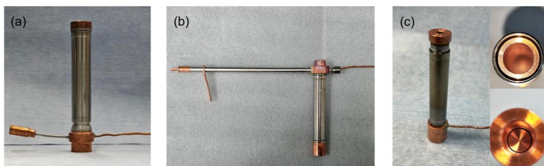
Figure 3. Photos of heat switches: (a) Active gas-gap heat switch with a short tail; (b) Active gas-gap heat switch with a long tail; (c) Passive gas-gap heat switch.
